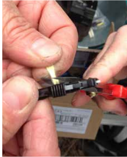
Aramid strength member captured by connector boot strain relief mechanism
